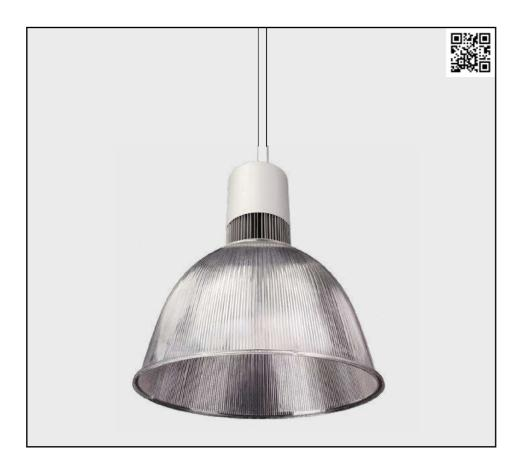
LED Pendant in industrial look, produced in die-cast aluminium. Supplied with Ø410mm prismatic polycarbonate shade. Suspension length 3m. Supplied with ceiling cup, also available in a 3-circuit track version. Equipped with Philips Fortimo LED module and Philips Xitanium LED driver.
