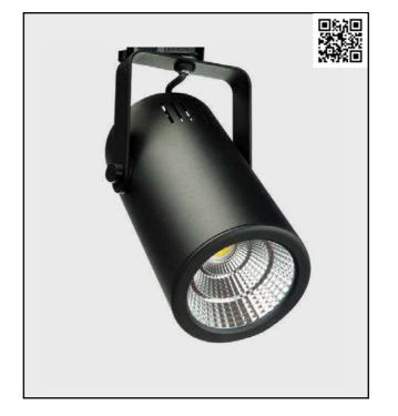
Tubular 3-Phase tracklight with built-in LED driver and aluminium die-cast heatsink. Powder coating finish. Glass standard included. Equipped with Philips Fortimo LED module and Philips Xitanium LED driver.
